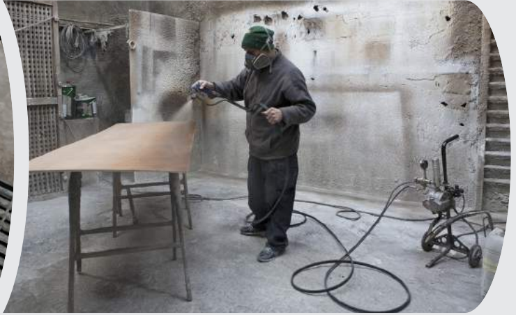
Wood varnish spraying.
